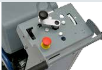
Threaded spindle with depth gauge
